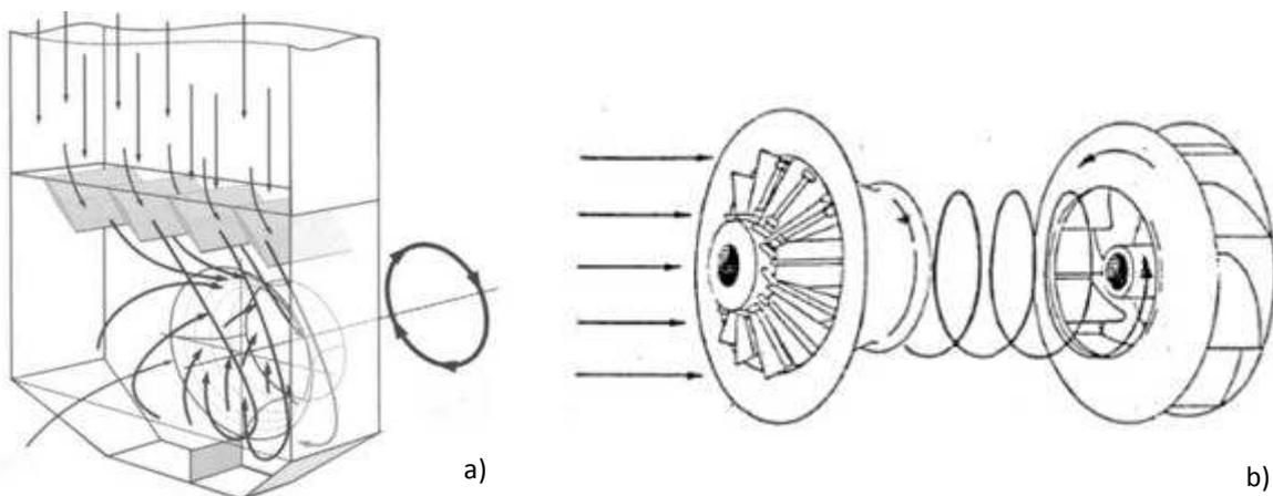
4. Inlet box damper whirl (a) and inlet vanes whirl (b)
