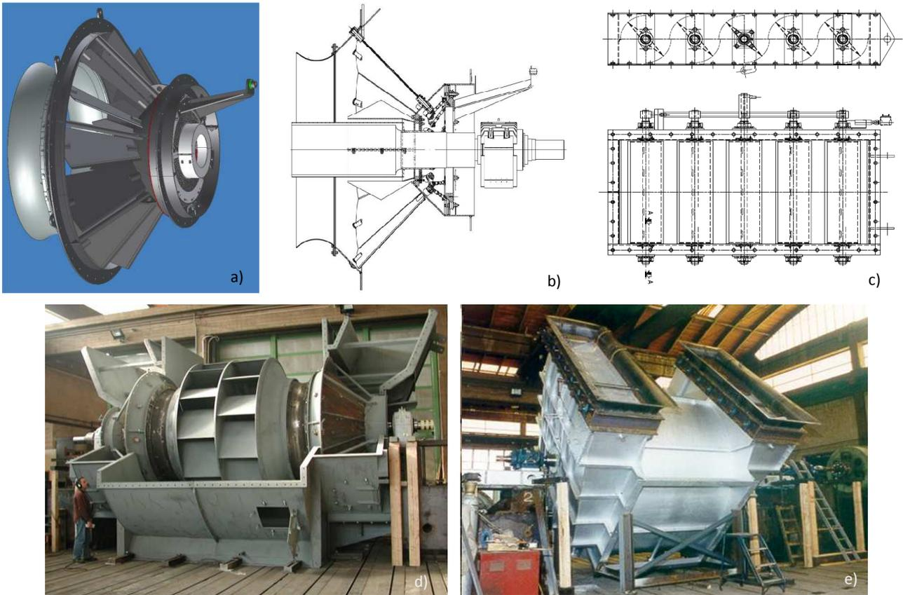
5. Variable inlet vanes (a,b,d) and Inlet Box Damper (c,e) drawings and pictures
