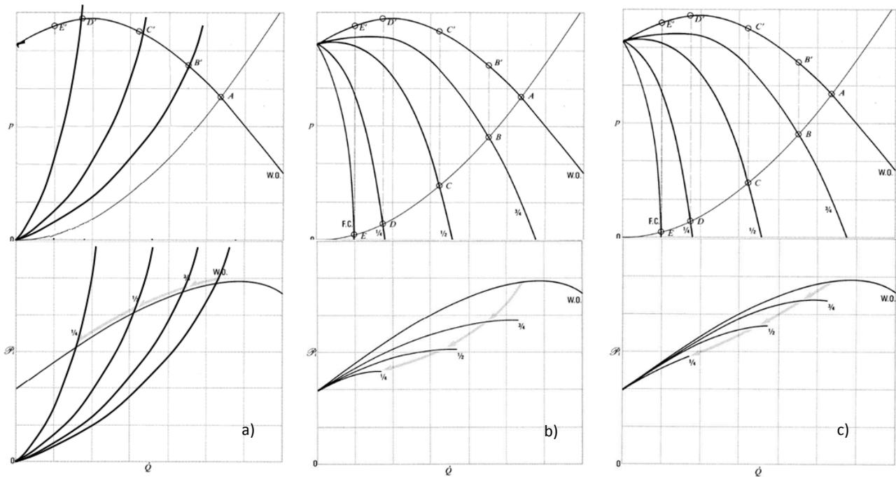
7. A type regulation device (a), Variable Inlet Vanes (b) and Inlet Box Damper (c) power reduction
