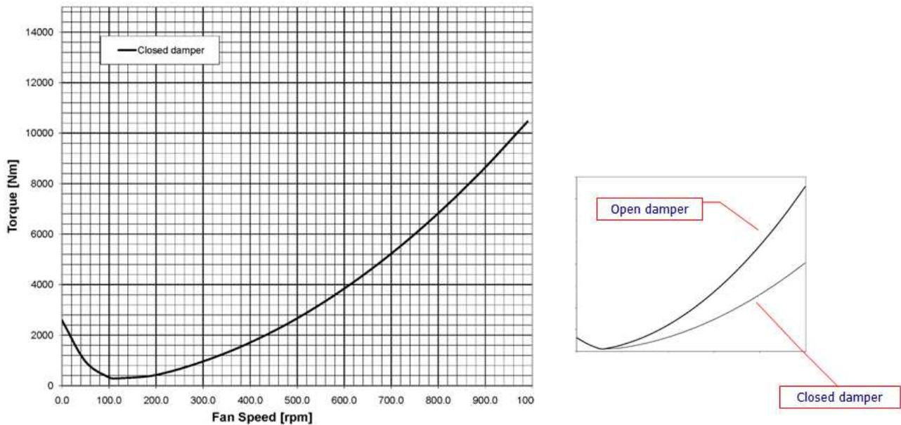
8. Start-up curve with closed or open throttling device
